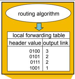
Routing algorithm *creates* the forwarding table, which is used on a per-packet basis
