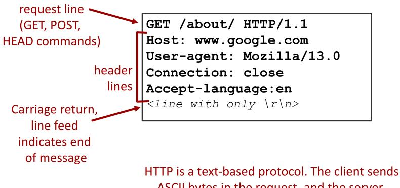
ASCII bytes in the request, and the server responds with ASCII bytes in the reply.
