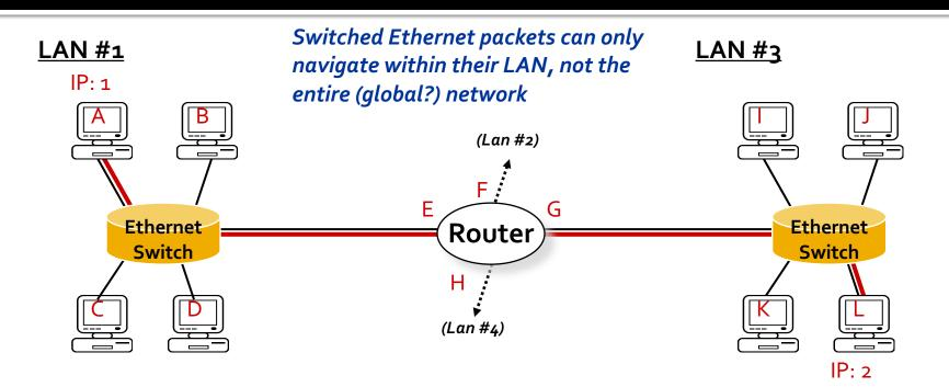
(1) A (1) transmits to L (2) using IP. Ethernet frame destination is <u>router</u>
